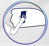
Apply 1st coat with putty blade. [Thickness of 0.5-1 mm]
