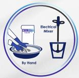
Add Putty in water to obtain a lump free paste & mix well. [Recommended mix 40% water]
